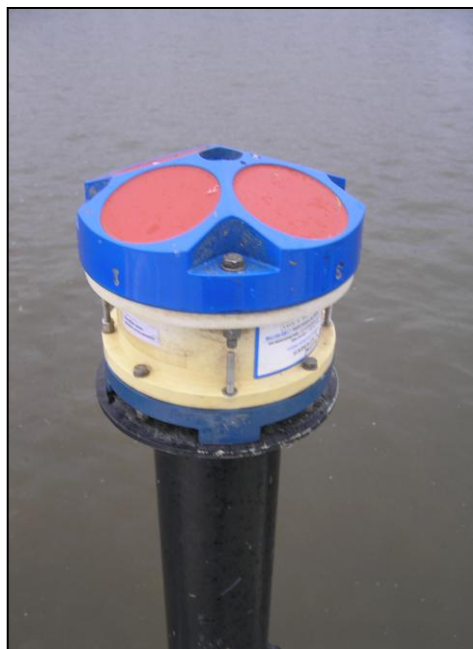
Fig. 3 Current meter ADCP WHM300-I-UG1
